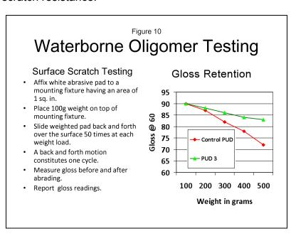
**Figure 10** describes the surface scratch test method used. The gloss retention was measured for loads from 100 g to 500 g in 100 g increments. At each load the sample received 50 abrasion cycles with a white abrasive pad (3M ScotchBrite). The control material had much poorer resistance to abrasion and showed a much more significant loss in gloss than the PUD 3 sample. PUD 3 maintained a relatively high level of gloss for the duration of the test.
