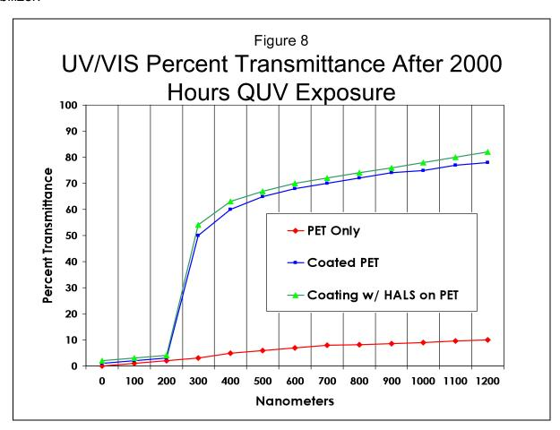
**Substrate Performance Observations:** Certain grades of PET will degrade when exposed to heat, light and moisture for extended periods. A properly formulated coating can lessen the degradation and provide a protective wear layer for the PET. The addition of HALS and light absorbers can further enhance protection.
