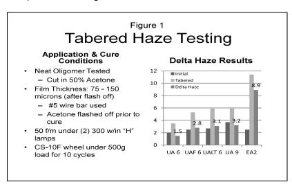
As these oligomers vary widely in viscosity, acetone was added to each to allow good control of film thickness. A photoinitiator (PI) was added to allow for UV curing. Each mixture was applied to a transparent substrate and UV-cured after removal of the solvent, yielding a dry film thickness of 75 microns. An epoxy acrylate (EA2) oligomer was also tested for comparative purposes.
