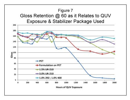
The coated PET without light stabilizers showed gloss retention of 70% of its original value, while the PET coated with the light stabilizer containing formulation retained 86% of its initial gloss after exposure. Finally, the uncoated PET performed very poorly and maintained only 3% of its initial gloss value.
